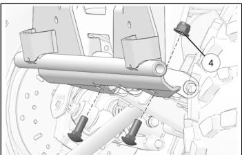
2. Drill 1/2" holes through the vehicle bumper.
