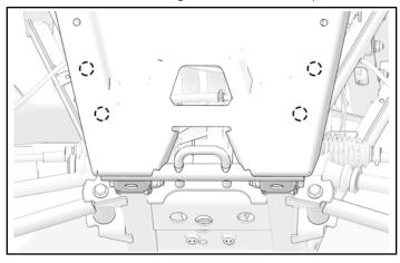
3. Install the four upper M10 screws ②, washers ⑥, and nuts ⑤.
